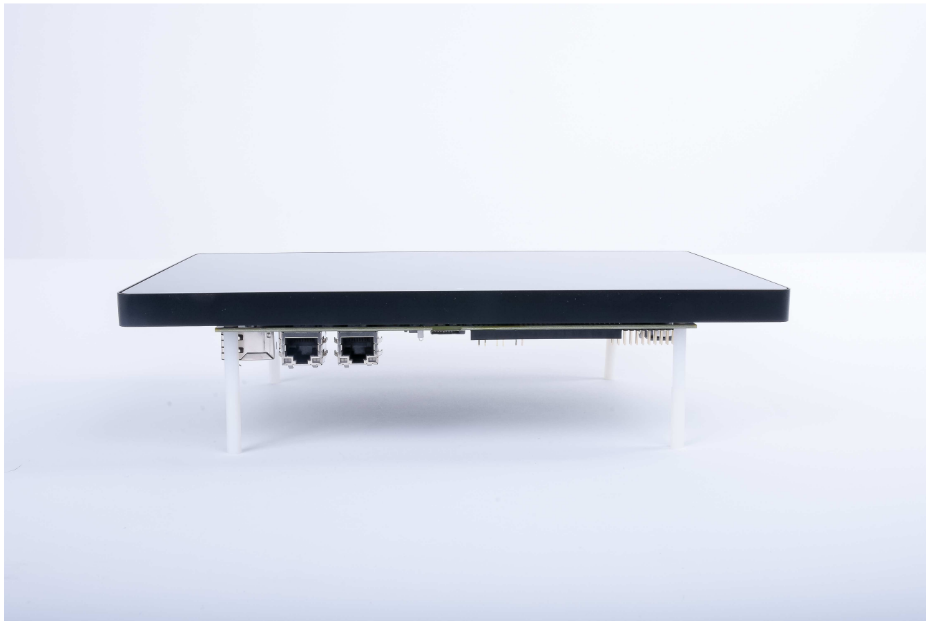
Figure 3. AM572x IDK EVM with LCD Display Assembly Attached - Top View
